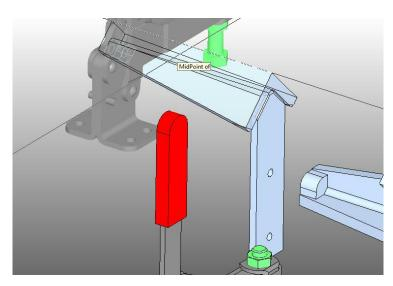
(the clamp will be "ghosted" as it is moved about – it may not appear to be at the intended location at times, but assuming the "from" position is correct initially, it will translate to the correct point after a suitable snap position is selected).
