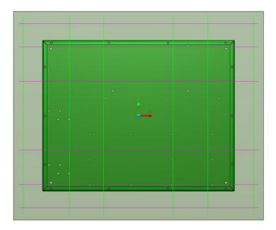
Lets assume that welds are needed on the external corners of the box. At the moment, the fixture lines will inhibit access on the outside of the box, so we will shrink them back:
