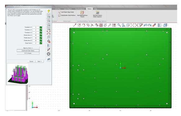
The part is now located at **X0 Y0 Z2** (the default position).
