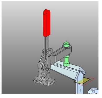
Based on the default entries in the Clamp Import Wizard page, some necessary boundary solids are created, along with the fixture blade position lines for the clamp.
