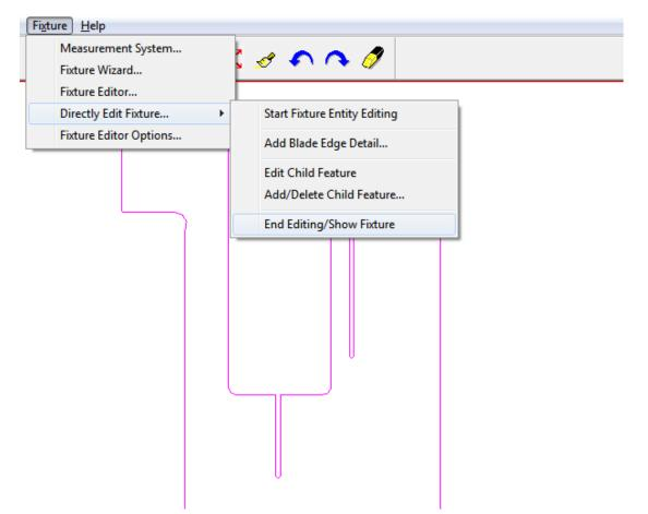
Once the fixture is updated, the blade will be regenerated with the changes (as long as the blade geometry is still a closed shape). The blade will be displayed in a slightly different hue to show it has been modified.
