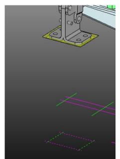
Finally, it is necessary to bolt the clamp and "clamp tower" to the base plate. Using the options below, the necessary locations are digistised:
