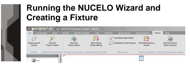
The "Fixture" icon set contains several entries: The first menu entry enables the system to be set to inch or metric. The second menu entry runs the NUCLEO Fixture Wizard that takes the user through a step-by-step process to design the fixture. The third option – "NUCLEO Fixture Editor" enables the user to go back and modify an existing fixture. Additional options are explained later.
