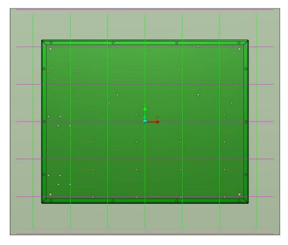
Because we defined a boundary, the boundary is considered when the fixture lines are calculated (unless when the boundary is created, we deliberately excluded it from being so). Note that the top-most and bottom-most magenta (horizontal) lines are not overlapping the green ones. This is OK, we will just move them in -Y and +Y respectively, and move the outermost green (vertical) lines in -X and +X respectively.
