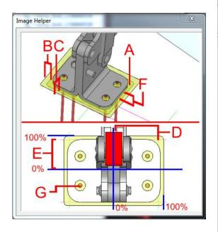
Fields **(B)** and **(C)** specify how much larger the fixture lines (to define the "clamp tower") should be, so to correctly encapsulate the clamp base. This is added to the oversize **(A)**.
