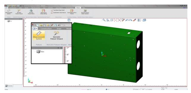
In the workspace, all the solid bodies found in the CAD file are listed. Generally, it is better to reduce the numbers of solids needed to create a good fixture, to reduce memory overhead and increase speed. Unsewn sheet bodies will also slow down the process, so a clean model is a good target.
