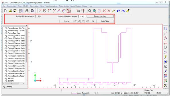
From this dialog, the process or direct editing can be started straight away, or before editing, the option to run a line/arc reduction on the blade is available. Once the "**Begin Editing**" button is clicked, the "Figure Edit" mode is started (this is apparent by the red box in the bottom right of the NUCLEO Fixture window):
