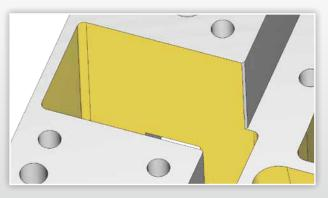
The WIRE Expert analyzes the imported 3D components for erodible geometries. The complete component can be interrogated or individual geometries or surfaces; edges can be selected manually.
