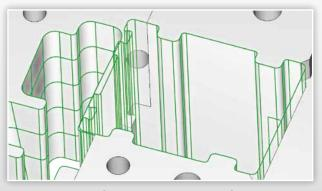
Machining profiles are suggested for the recognized features. The User has the option to use customized machining schemes that check the color of the feature's faces, to assign preset machining technology.
